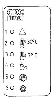
1. Lights up in red if the sensor in the cooling system senses a too high temperature. The whole unit will then be switched off. This function assures the compressor against break-down.
